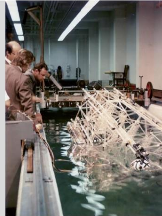
Installation procedures were then tested in laboratory tanks
